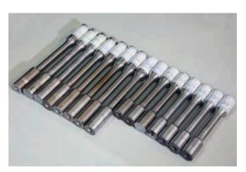
Precision machined test bars in accordance with ASTM A-370
