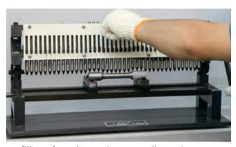
Profiling of test bars prior to tensile testing
