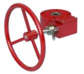
This operator is excellent for the safe handling of spring return actuators. During pneumatic operation, the worm of the gear unit is disengaged. Should the valve require opening or closing in the event of power loss, manual rotation of the declutch lever will provide a camming action and engage the worm to the segmented worm gear, allowing rotation of the valve using the handwheel.
