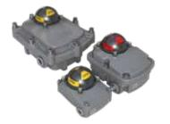
Provide visual and electrical indication of position on any VDI/VDE 3845 compliant quarter-turn rotary actuators. The VSMs can be installed in both perpendicular and parallel orientations without changing brackets. Available as general purpose (Series 5A and 5B) or hazardous locations (Series 5C Explosion Proof, and 5A/B Intrinsically safe).
