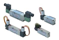
These units can be used with either spring return or double acting actuators where on/off electrical operation is required. Units have 1/4" NPT conduit connections and DIN units have cable gland PG9 connectors, also available with 1/2" NPT conduit adapters.
