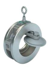
Rite's Bray/Rite wafer combination swing check valves are flowactivated and Rite Sized. Bray/Rite inlet ports and disc have been shape optimized to achieve a fully open position at low flow rates (3 ft/s on average). Therefore, the Bray/Rite operates exceptionally well in the flow rates typically found in pipelines containing control valves and lines with varying media flows.
