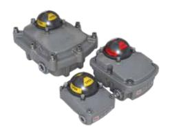
Series 5A, 5B and 5C Valve Status Monitors (VSM) provide visual and electrical indication of position on any VDI/VDE 3845 compliant quarter-turn rotary actuators. The VSMs can be installed in both perpendicular and parallel orientations without changing brackets. Available as general purpose (Series 5A and 5B) or hazardous locations (Series 5C Explosion Proof, and 5A/B Intrinsically safe).
