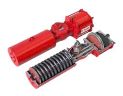
Series 98 scotch-yoke actuator features a modular design with a wide range of modules to suit the required process application. The heart of the Series 98 is the yoke, available in symmetrically or canted, that converts linear motion into rotational motion.
