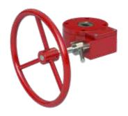
This operator is excellent for the safe handling of spring return actuators. During pneumatic operation, the worm of the gear unit is disengaged. Should the valve require opening or closing in the event of power loss, manual rotation of the declutch lever will provide a camming action and engage the worm to the segmented worm gear, allowing rotation of the valve using the handwheel.
