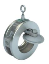
Rite's Bray/Rite wafer combination swing check valves are flow-activated and Rite Sized. Bray/Rite inlet ports and disc have been shape optimized to achieve a fully open position at low flow rates (3 ft/s on average). Therefore, the Bray/Rite operates exceptionally well in the flow rates typically found in pipelines containing control valves and lines with varying media flows.
