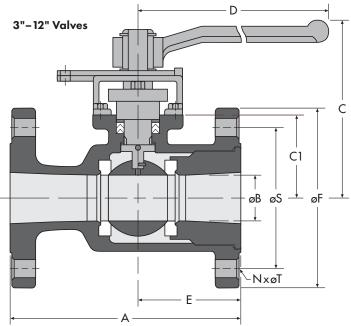
**NOTE:** Gear Operators are suggested on size 10" and 12" valves. **NOTE:** A trunnion-like Ball Support is included on size 12" valves.
