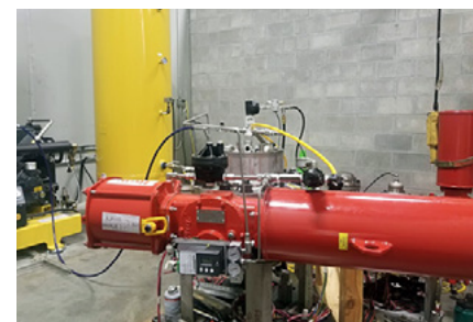
Test setup where the McCannalok S42 High Performance Butterfly Valve and S98 Scotch Yoke Pneumatic Actuator achieved more than 1 million cycles with zero leakage.
