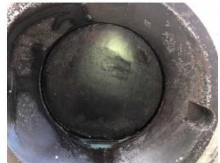
After 18 months in service with no issues, the valve showed no signs of wear or upstream media buildup.
