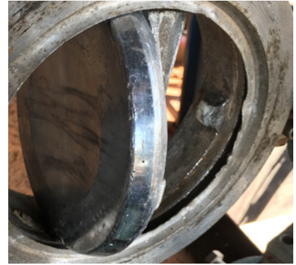
The existing butterfly valves showed frequent signs of damage from the harsh media, requiring shutdowns every 2 weeks for cleaning and repair.
