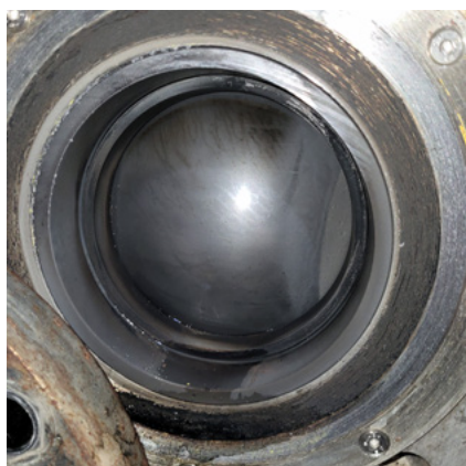
After 18 months of service, Bray's Series 19L segmented ball valve showed no signs of wear or damage.
