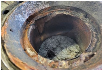
Competitor ball valve showed signs of severe damage to ball (left) and seat (right) caused by abrasive media.
