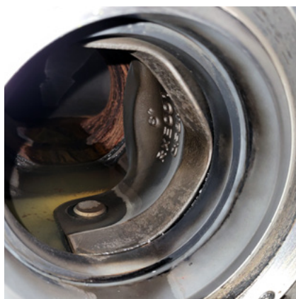
After 18 months of service, Bray's Series 19L segmented ball valve showed no signs of wear or damage.
