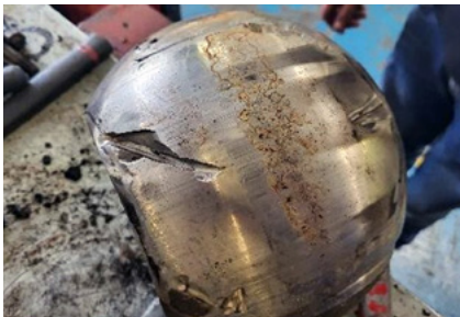
Competitor ball valve showed signs of severe damage to ball (left) and seat (right) caused by abrasive media.
