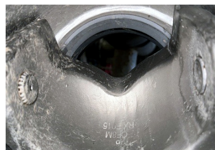
After 24 months in service, inspection of the S19L showed no signs of erosion on the ball segment, seat, body walls, or liner.
