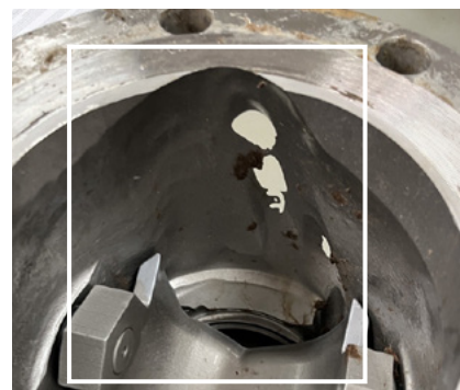
Inspection of a competitor's failed control valve shows signs of extensive erosion of the body wall, segment, seat, and flange area.
