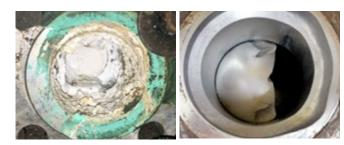
**CHALLENGES**: Typical valves show extreme solids buildup or accelerated erosion after only a few months of service in harsh sugar processing applications.
