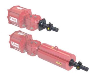
Hydraulic Dampener - Series 98 scotch yoke actuator option provides adjustable cushion before valve seating preventing slamming and seat damage to the valve and vibration shock to the piping.
