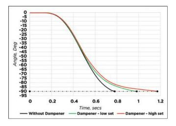
Operating Time vs. Angle of Disc Rotation, Without and With Dampener (Example: Tri Lok Triple Offset Valve with Series 98 Spring-Return Pneumatic Actuator).
