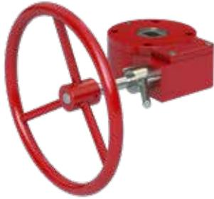
This operator is excellent for the safe handling of spring return actuators. During pneumatic operation, the worm of the gear unit is disengaged. Should the valve require opening or closing in the event of power loss, manual rotation of the declutch lever will provide a camming action and engage the worm to the segmented worm gear, allowing rotation of the valve using the handwheel.
