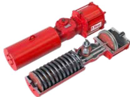
Features a modular design with a wide range of modules to suit the required process application. The heart of the Series 98 is the yoke, available in symmetrically or canted, that converts linear motion into rotational motion.
