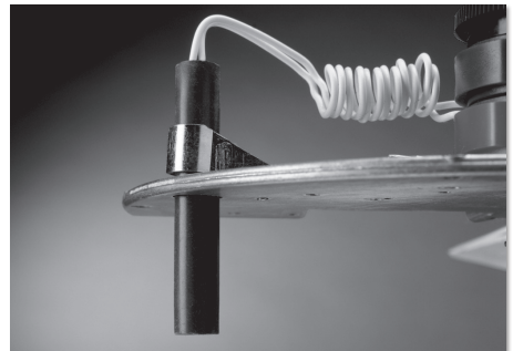
Figure 10. Heater installed on an S70 switch plate.
