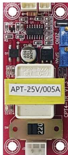
Figure 30: Analog position transmitter.
