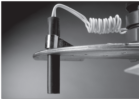
Figure 12. Heater installed on an S70
