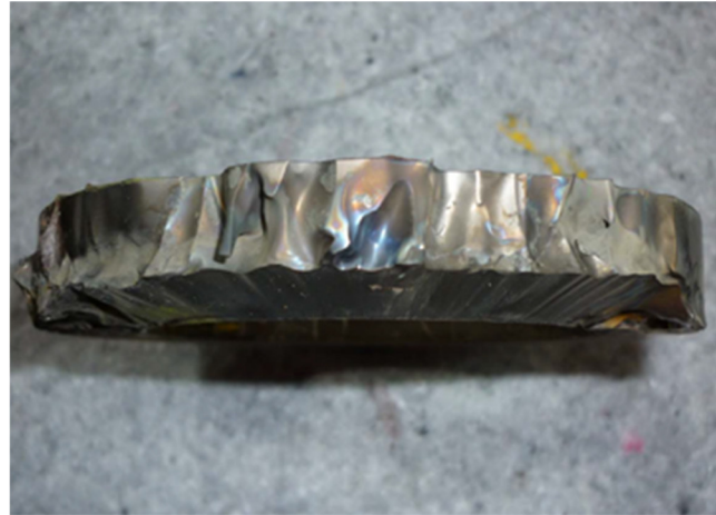
Erosion due to high velocity flow
